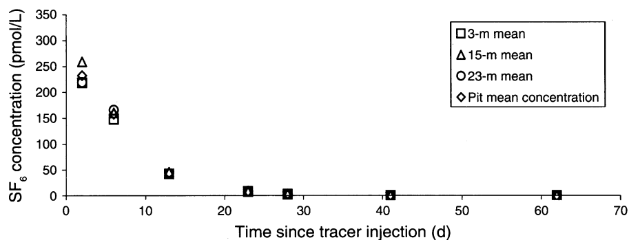
FIG. 15. Time series of \text{SF}_6 concentration in Herman Pit as a function of time in days since injection on 9 September 1998.
